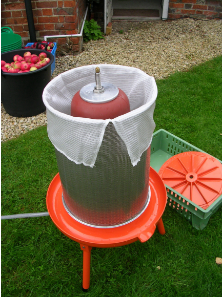
Figure 3. Press with the lid removed showing the brown rubber membrane and porous fabric liner.
