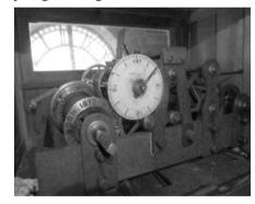
The clock is adjusted by a lever on the mechanism, but in reverse to the clockface. Fine adjustment is made by a collection of lead weights, a small nut, copper pennies and also a screw collar on the end of the pendulum. Make the pendulum shorter it runs faster and longer slower. Fortunately this adjustment is rarely needed and
